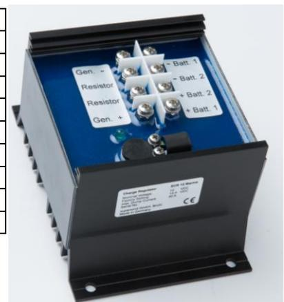
LED indicating that max. charging voltage has been achieved (batteries fully charged)
