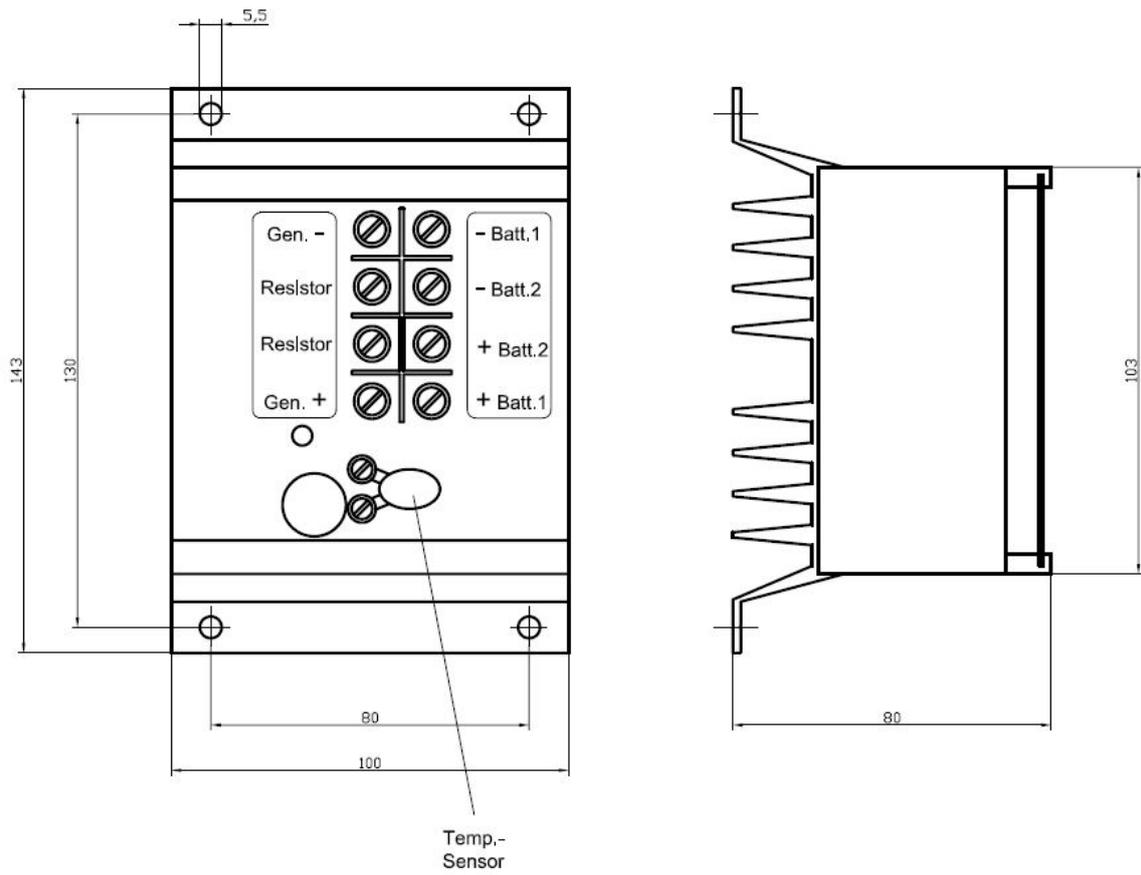
**Dimensions of the power resistor:**
